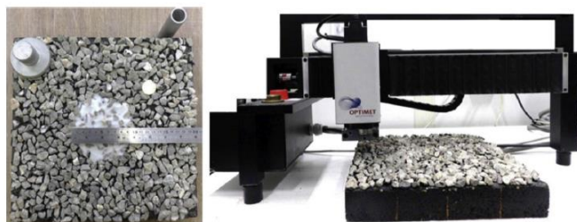
Fig. 4. Sand height (left) and laser profilometer measurements (right).
