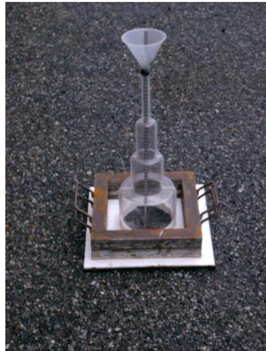
Fig. 2. Example of falling head test on porous European mixes.
