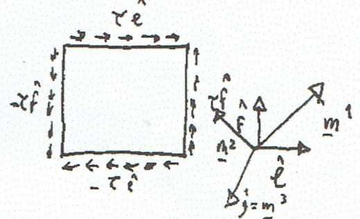
Allora dall' (10) si ha: a)  $\underline{\underline{\tau}} \underline{\underline{m}}^1 = \lambda_1 \underline{\underline{m}}^1 \Leftrightarrow \begin{pmatrix} \gamma m_2 \\ \gamma m_1 \\ 0 \end{pmatrix} = \begin{pmatrix} \gamma m_1 \\ \gamma m_2 \\ 0 \end{pmatrix} \Leftrightarrow \begin{pmatrix} \gamma m_1 \\ \gamma m_2 \\ 0 \end{pmatrix} = \begin{pmatrix} \gamma m_1 \\ \gamma m_2 \\ \gamma m_3 \end{pmatrix}$  cioè
